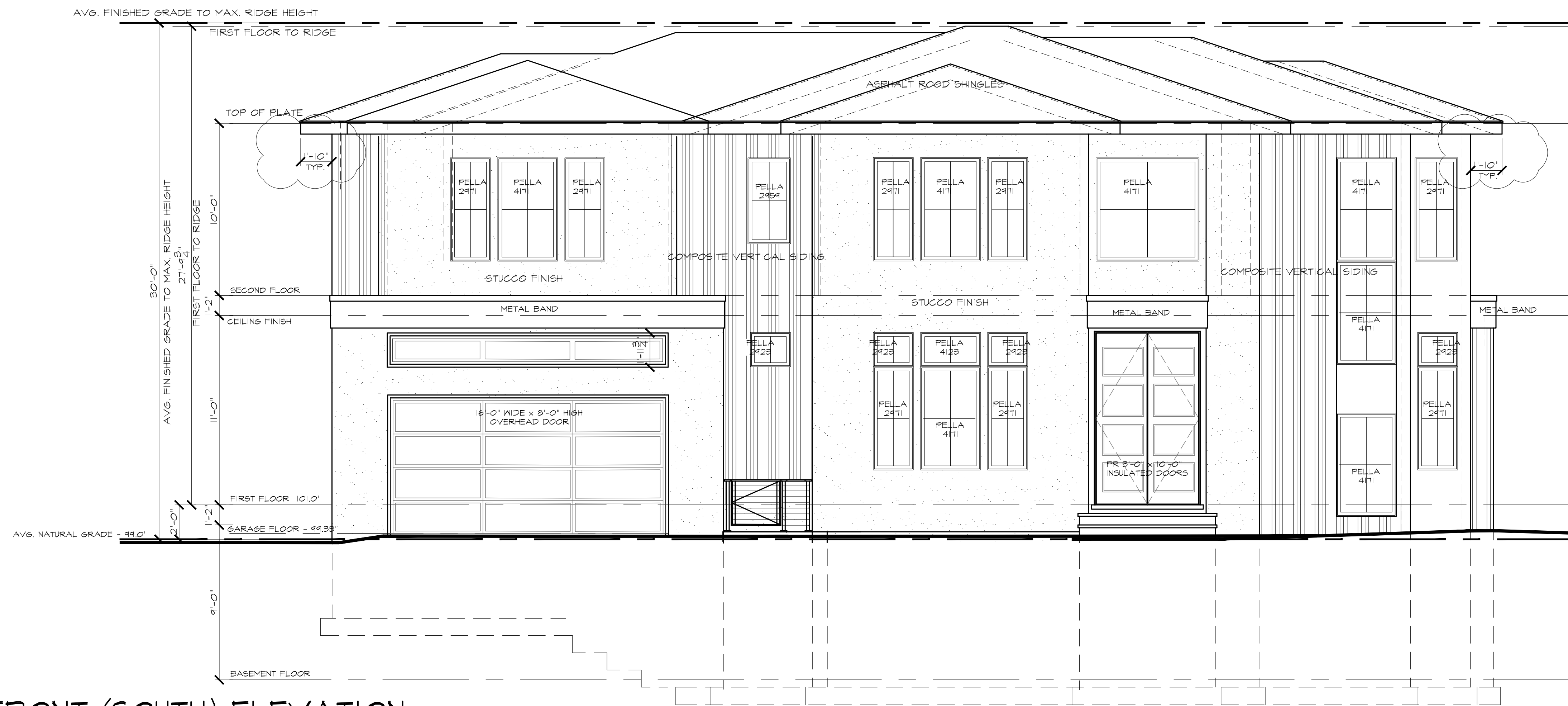
FRONT (SOUTH) ELEVATION SCALE: 1/4" = 1'-0"
