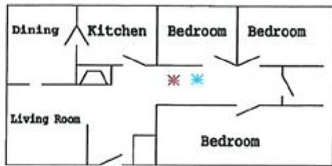
Figure 1 * Smoke Detector and Carbon Monoxide Detector needed
